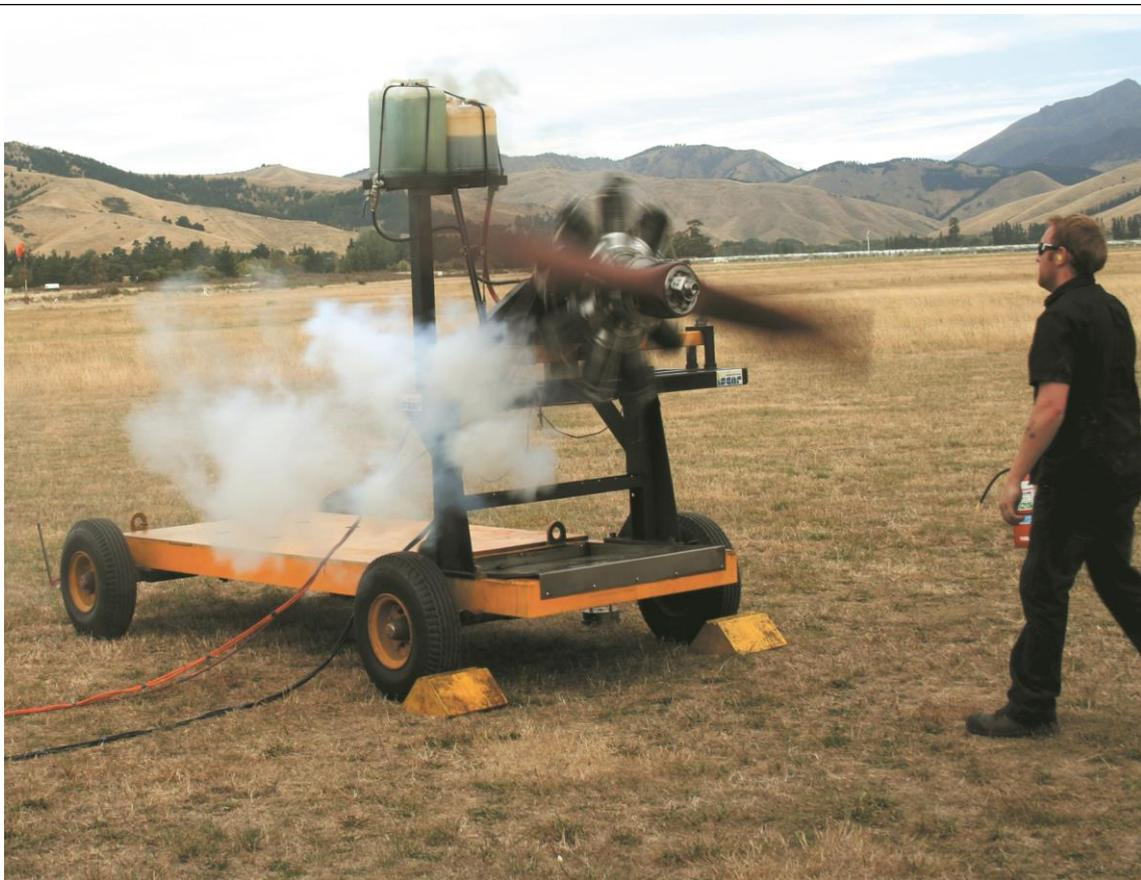
CAMS Engineer Dan Melling fires CAMS Gnome Rotary Serial Number CAMS 001 into life.
